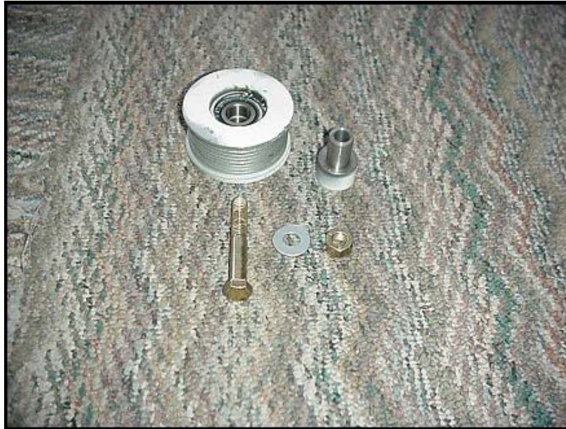
The real long term solution—A Grade 8 7/16" bolt—old spacer style or new, makes no difference if you upgrade the bolt size
